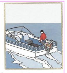
Assuming your steering system has frozen, control can be regained by disconnecting the "\_\_\_\_\_\_ - \_\_\_\_\_" fitting located by the engine & lashing an oar to the engine, as shown above.
